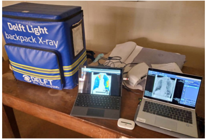
Delft Light ultra-portable X-ray machine and CAD4TB offline implementation set up for TB screening in Uganda.
